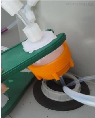
**Figure 11: Sample box filter housing**
